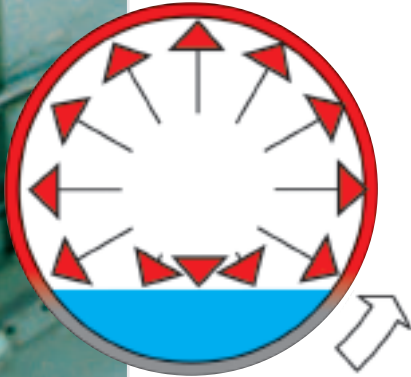
At low speed, condensate puddles in the bottom of the dryer.
